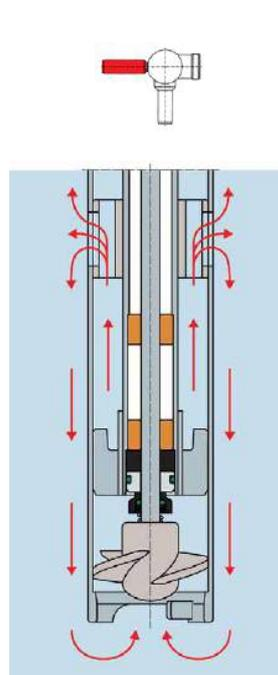
Outlet closed, mixing openings opened.
