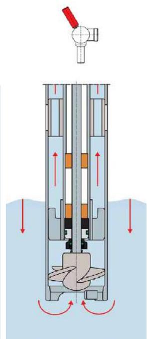
Outlet opened, mixing openings closed.
