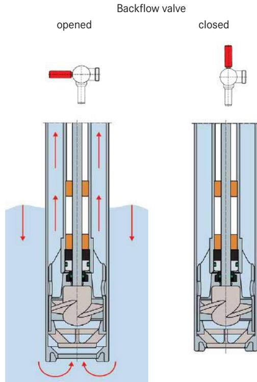
After pumping (left) the backflow valve is closed to remove the pump. The medium remains in the pump (right).
