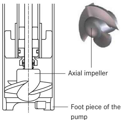
F/FP 430 with mechanical seal and axial impeller
