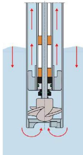
The mechanical seal prevents medium from getting into the inner tube while pumping.
