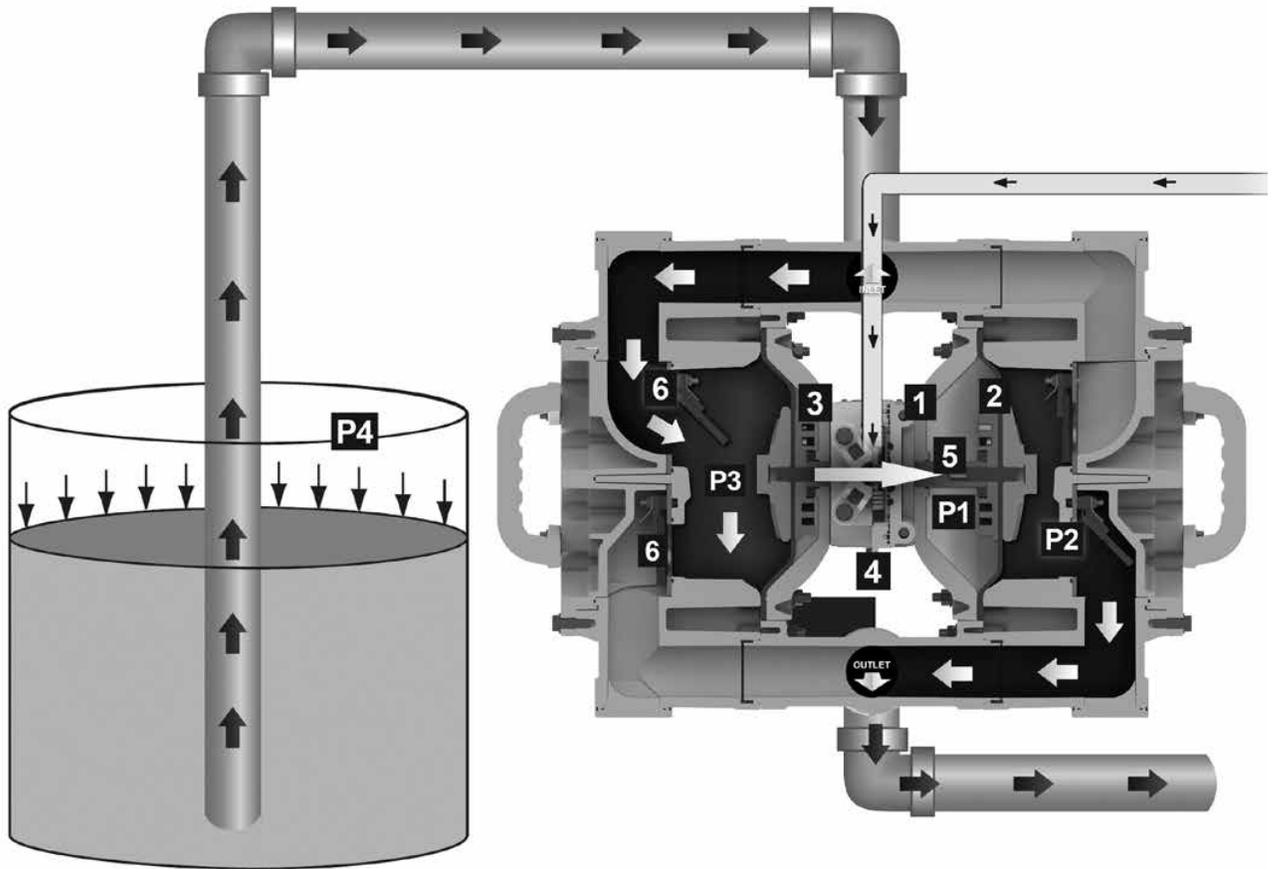
Gas-Operated Double Diaphragm (GODD) pumps are powered by compressed air or nitrogen.
